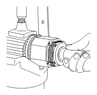
STARTING-MOTOR ASSEMBLY Assembling multi-plate clutch Screw intermediate bearing (1) to clutch housing (2). Always use new, microencapsulated hexagon bolts (3) of strength class 10.9. Use torque wrench. Slip thrust washer (4) onto intermediate bearing. Torque wrench: comm. avail. Tightening torque: 7...8,5 Nm
